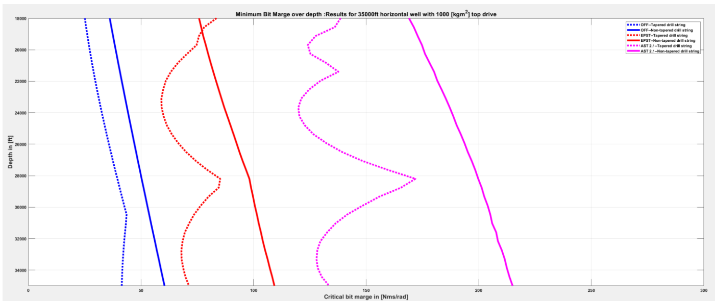
Figure 7: Comparison between various soft torque systems and drill string configuration for (top) drive inertia of 1000 [kgm 2 ]
