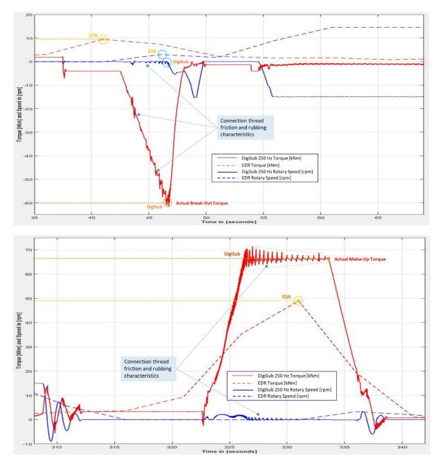
The showed in thread friction and rubbing phenomena are the signature for a healthy connection. Al and ML tools can use these patterns to recognize problems with the connection before the stand is used.
