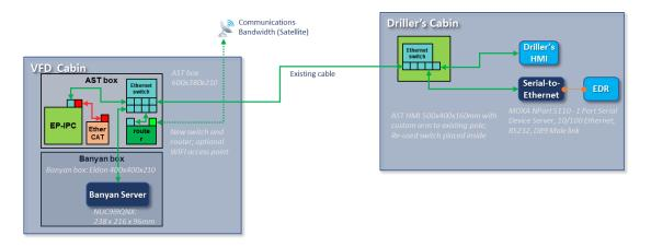
For the pilot, SigmaStream/Electroproject will install an Edge server to deploy Banyan applications. The Banyan Server will consist of two IPC's. One the DigiSub-AST IPC, hosting the Banyan DigiSub connection with the top drive PLC and VFD and one hosting the Banyan platform itself.
